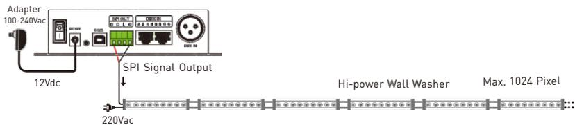
6.3 Connected with DMX 512 computer console to realize DMX decoding function.
