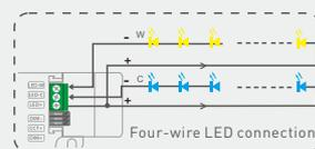
\* Adopting constant power program design, it keeps the same brightness in color temperature dimming, twice the rated power load can be connected.
