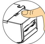
Break off the bottom left and right to remove the protective cover.
