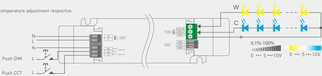
4. Brightness and color temperature adjustment simultaneous.
