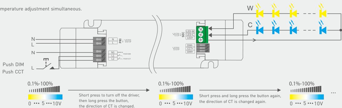
\* Dimming interface priority: First 0-10V, next Push DIM/CCT.
